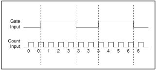
Figure 6. Gate Source Set to External Gate Input
